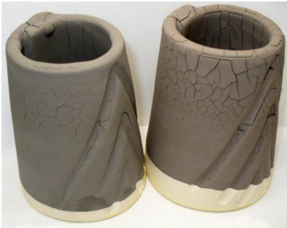
Cracks in the glaze surface before firing is a good indicator that your glaze application is too thick and may crawl
